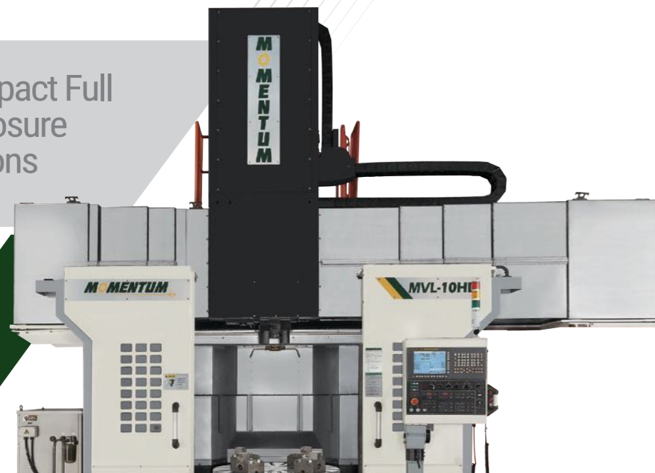
Enclosure's deep way covers meet doors, prohibiting coolant escapement.
